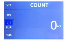
**NOTE:** When MIX & SINGLE modes are selected, the device verifies the BankNotes by images, MG, UV and DB (double notes detection). CNT mode has only DB detection.
